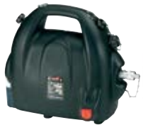
Battpac® LT Pump 350 kcmil AL. The battery-powered hydraulic pump, rated for 10,000 psi. Portable power for all Color-Keyed hydraulic heads, using just one Ni-MH 24V rechargeable battery.
