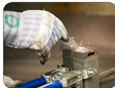
Step 6: Ignite material located on top of the lid using a flint igniter (FLTIG).
