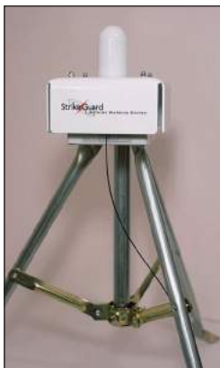
Lightning Warning System
