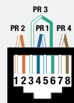
EIA/TIA568B AT&amp;T 258A WIRING
