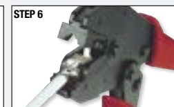
Crimp plug with the specially designed HTS2700 crimp tool.
